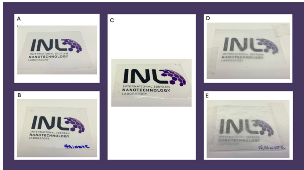
Fig. 4 The figure shows digital images of the control materials and those coated with sodium alginate solution. A Polystyrene substrate — control. B Polystyrene substrate coated with sodium alginate solution. C Film of sodium alginate solution. D Parchment paper — control. E Parchment paper coated with sodium alginate solution
