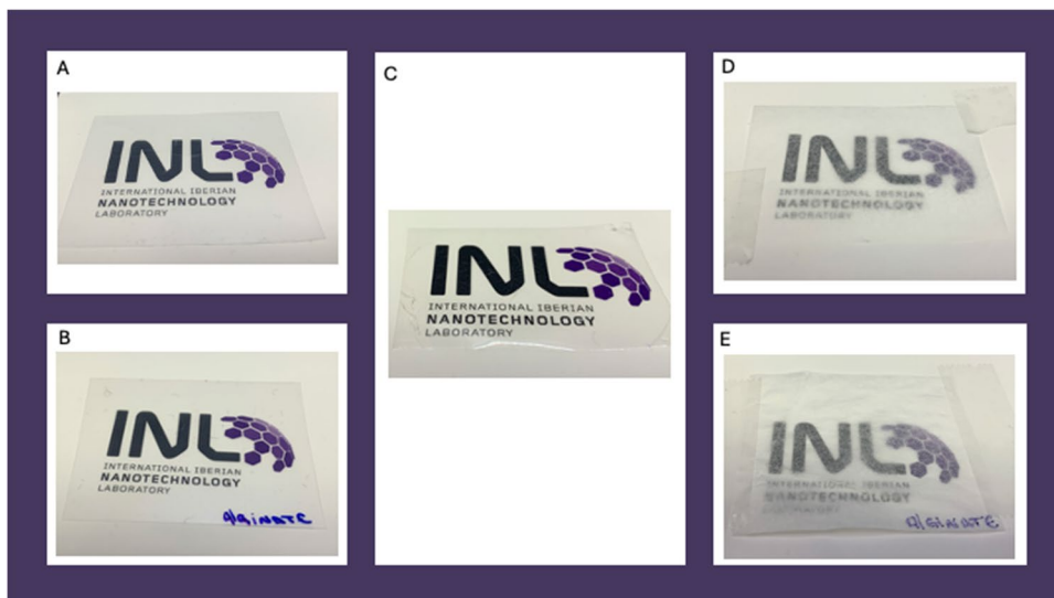
Fig. 4 The figure shows digital images of the control materials and those coated with sodium alginate solution. A Polystyrene substrate — control. B Polystyrene substrate coated with sodium alginate solution. C Film of sodium alginate solution. D Parchment paper — control. E Parchment paper coated with sodium alginate solution
