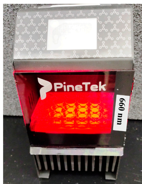
Figure 5. Diagram of the experimental irradiation setup used for photodynamic therapy (PDT). Irradiation was performed with a PineTek Biotable®—PINETEK LLC, College Station, TX, USA, a red light-emitting diode (LED)-based device that consists of 24 emitting centers with a wavelength of 660 nm. LED arrays were arranged so that each LED array was placed under a well from the well plate, providing the same average irradiation. The RSD values of irradiance obtained with this device were 75 mW/cm 2 . Variation from well to well remains at about 10%. The configuration allows for consistent and homogeneous light exposure, ensuring reproducibility of the photoinactivation experiments. The light dose applied was 15 J/cm 2 at an exposure time of 3 min 20 s. In opposite to illuminating a single well each time, the device is more precise and reproducible.
