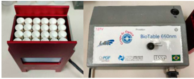
Fig. 6. The (Left) plate holder and LED array along with (Right) LED driver and power controller.
