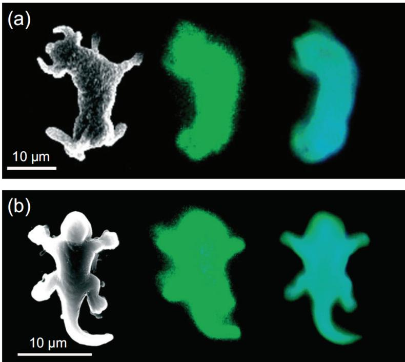
FIGURE 3 Scanning Electron Microscope (left) and Fluorescence Microscopy images of three-dimensional (a) microbull and (b) lizard fabricated from different resins (center and right). Reprinted with permission from (Sun, Z.B. *et al.*, 2008). Copyright (2014), John Wiley and Sons, Copyright Clearance Center.
