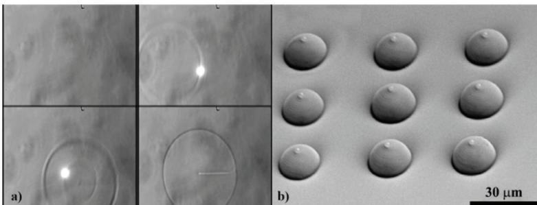
FIGURE 4 (a) Screenshots of the real-time lens fabrication (radius 25  $\mu\text{m}$ , height 8  $\mu\text{m}$ ). (b) SEM micrograph of a microlens array with 15  $\mu\text{m}$  diameter. Reprinted with permission from (Malinauskas *et al.*, 2010). Copyright (2014), IOP Publishing. Reproduced by permission of IOP Publishing. All rights reserved.
