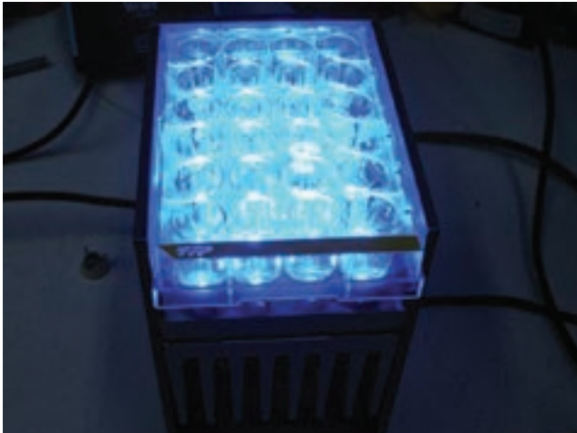
PDT for superbugs: In vitro experiment using curcumin as the photosensitizer and 450-nm LED illumination for antimicrobial PDT. Courtesy of C. Kurachi
